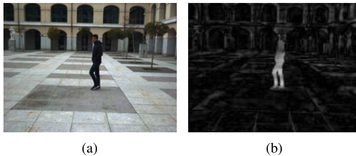
Fig. 9.2 Original camera image from the Emergency Stop scenario (a) vs. corresponding direct reconstruction error image (b).
