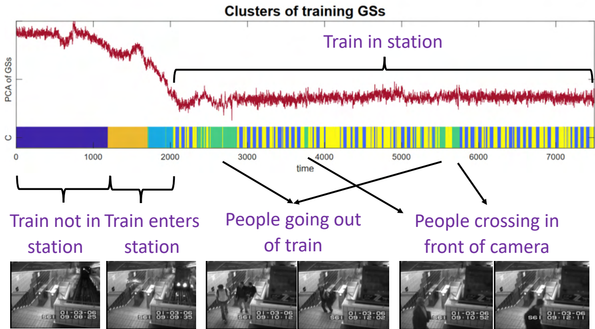
Fig. 5.15 First component of the PCA of the training GSs in subway Exit dataset, and corresponding color-coded clusters assignment (C), with examples of related images. © 2021 IEEE.
