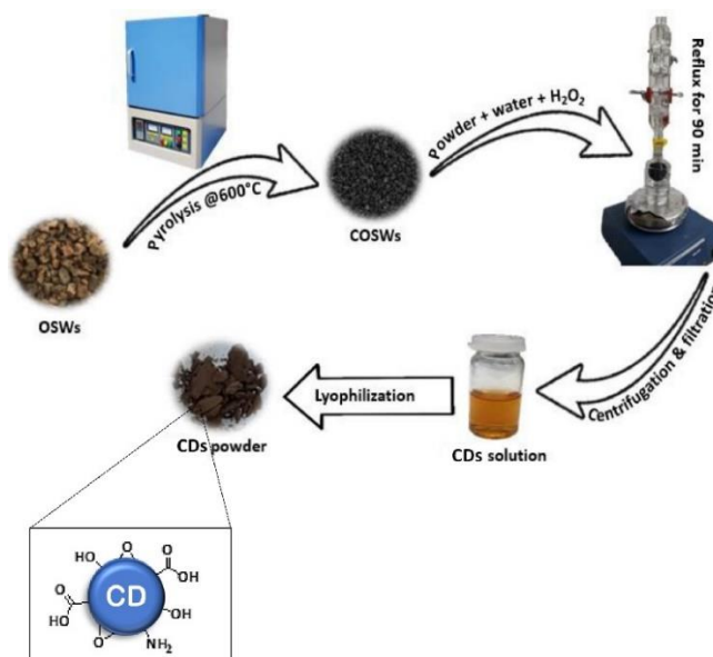
Fig. 3 Schematization of the synthesis process of CDs.
