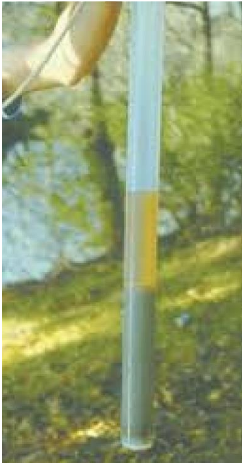
Figure 16: Bailer just extracted from a well. The liquid exhibits a clear separation between two distinct phases. At the bottom, you can observe groundwater, which appears particularly turbid, with a significant level of opacity. Overlying this aqueous phase there is a layer of floating hydrocarbon product, known as NAPL (Non-Aqueous Phase Liquid).
