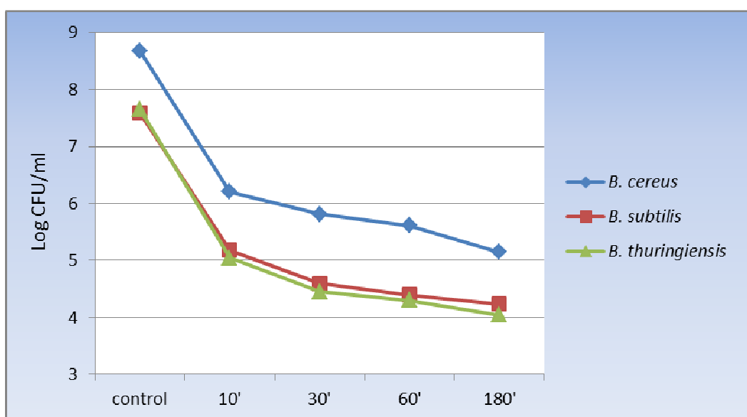
Figure 3: Log reduction of Bacillus cereus , B. subtilis and B. thuringiensis after 10 to 180 min of exposure to 1 ppm of ozone.
