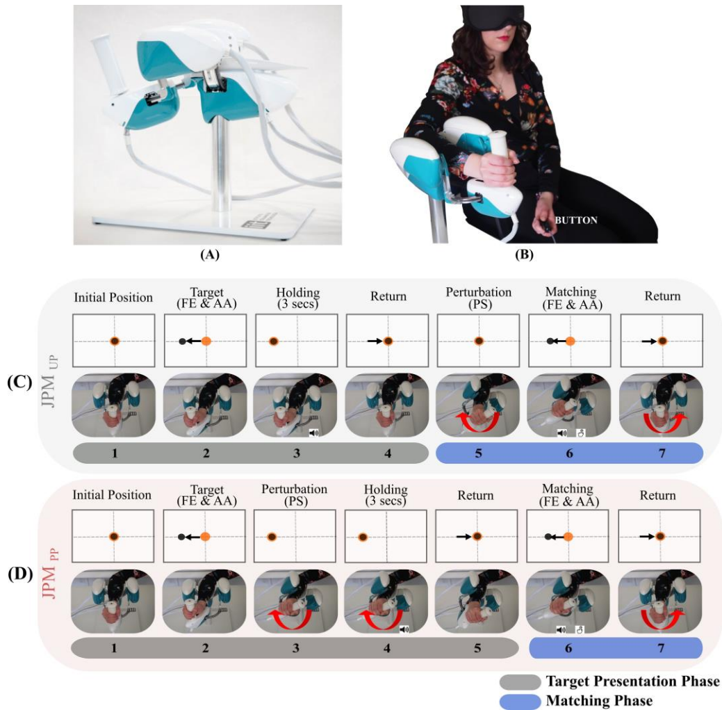
Figure 12: (A) Experimental setup. The subject is comfortably seated on a chair with the right forearm fixed on the Wristbot robotic device while holding its handle. In the contralateral hand the subject holds the button to press during the proprioceptive "Matching Phase". The subject wears a mask over his eyes to perform the experiment based only on his proprioceptive feedback. In the panel (B) and (C) are represented the temporal sequences for the two JPM conditions: JPM UP and JPM PP . From the initial position the wrist joint is passively moved towards the proprioceptive target (passive reaching) and then maintained for three seconds. An auditory cue marks that the proprioceptive target is reached. After returning to the resting position participants are asked to match the target, as accurate as possible (Matching Phase) by pressing the button with the contralateral hand. Another auditory cue signals to the subject the start of the Passive Matching Phase in which it is required to stop the robot once the same movement amplitude has been perceived. In different temporal moments, depending on the condition experienced, a perturbation is given (angular rotation along the PS axis of a certain random amplitude). This is evidenced by the red arrow in the figure. Orange dot represents the device end-effector position, while the black dot represents the proprioceptive target position.
