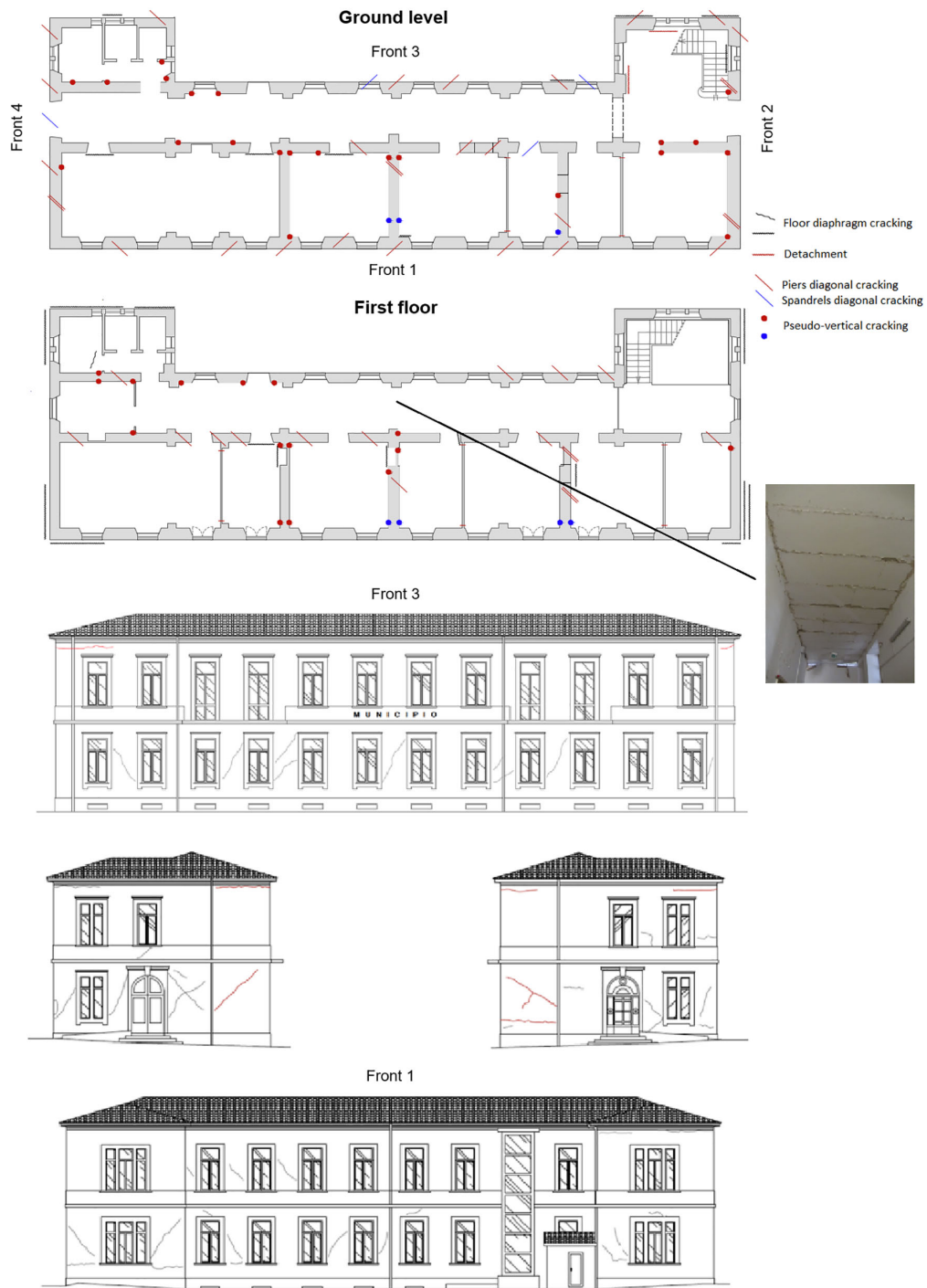
Figure 3.10: Pictures and schematic representation of the internal structural damage and external cracking pattern surveyed on the Pizzoli town hall building in June 2017, after the seismic sequence of earthquakes that hit Central Italy at the end of 2016.
