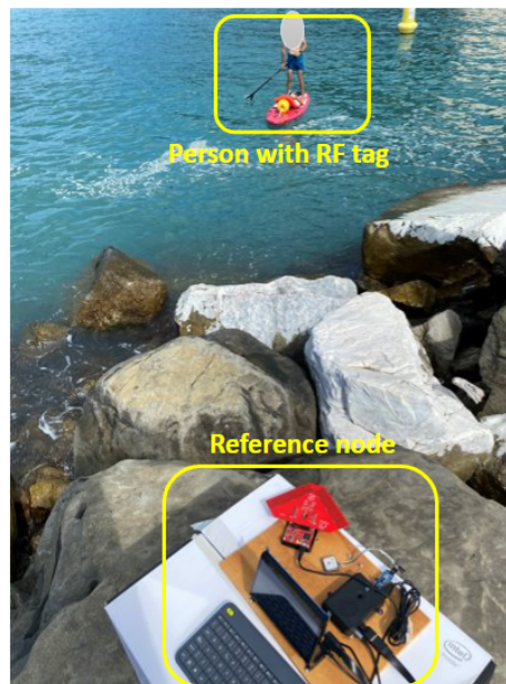
Figure 3.16: Experimental setup: Outdoor Scenario 2
