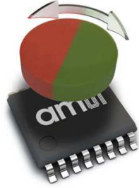
Fig. 2.4 Typical arrangement for placing the rotating magnet close to the sensing surface of the AS5045 chipset. Source: Microsystems [2017]
