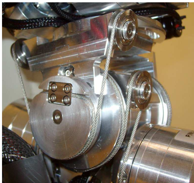
Fig. 2.7 Close-up view of the waist differential drive. Source: Tsagarakis et al. [2006]
