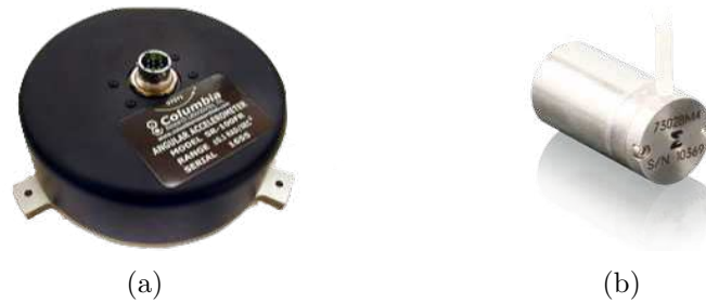
Fig. 4.1 Three-axes direct sensing angular accelerometers: (a) fluid rotor model SR-100FR by Columbia Research Laboratories, providing high sensitivity from 0.1. Source: https://www.crlsensors.com ; (b) piezoresistive model 7302BM4 by MEGGITT, of much smaller dimensions, but with lower sensitivity ( 5\text{mV} per \text{krad s}^{-2} ). Source: http://www.akron.be .
