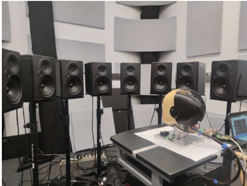
Figure 8.2 Impulse Responses Measurement Setup
