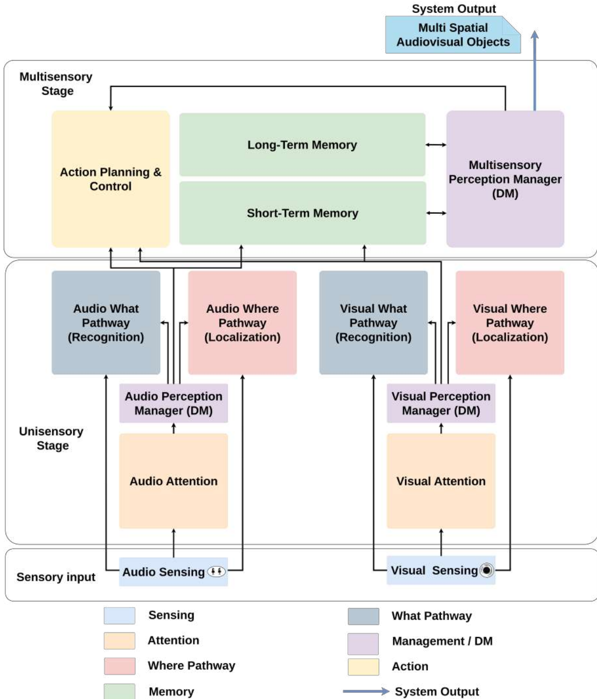
Figure 5.1 The Overall Structure of The General Audio-visual Proposed Perception Architecture.
