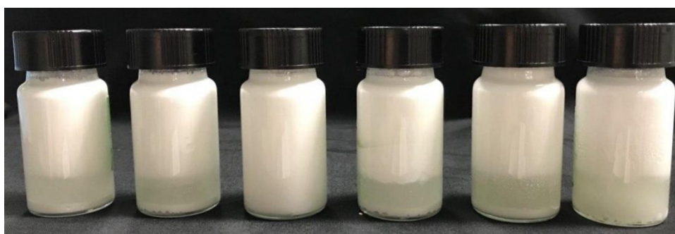
Figure 9. Prepared PLA-based emulsions using different surfactants from left to the right: Tween ® 80- Span ® 20- Tween ® 65- Span ® 65- Tween ® 85- Mixture of Span ® 20:Tween ® 80 in the total weight percentage of 60:40.
