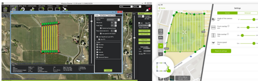
Figure 3-4 GCS software for photogrammetric flight plans: Mission Planner on the left and pix4dcapture on the right
