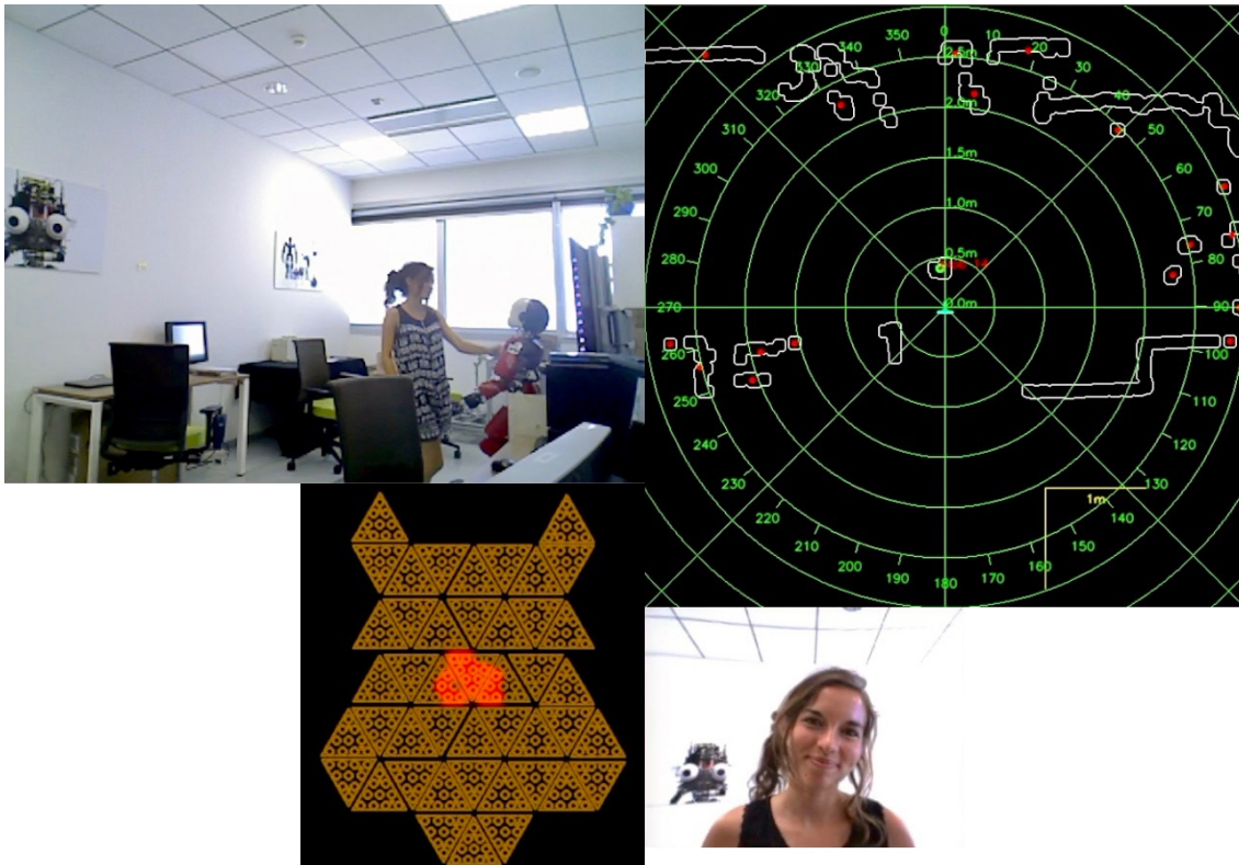
Figure 3 - Sensory information: top left – experimental room with a participant; top right - laser radar tracking the participant; bottom left - iCub's torso skin sensing touch; bottom right - iCub tracking the participant.
