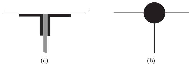
Figure 1.2: Reinforced-shell structure (a) and related semimonocoque simplification (b)
