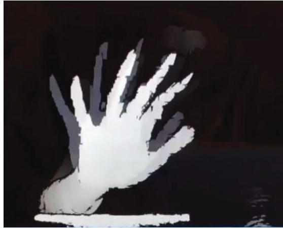
Figure 2.17: Artifacts in the depth estimate of a moving hand acquired by the Intel RealSense F200 depth camera. The depth of the moving hand should only be the brightest silhouette, however a shadowed hand appears in the estimated depth map.
