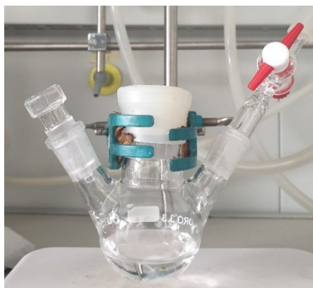
Figure 2.25. Setup for the synthesis of acetalated dextran.
