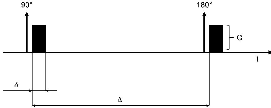
Fig. 2.3: Pulsed gradient spin echo acquisition sequence. It is composed by two radiofrequencies at 90^\circ and 180^\circ and two gradient pulses just after them. The two gradient pulses are characterized by a duration \delta and a strength G , while \Delta is the time occurring between them.
