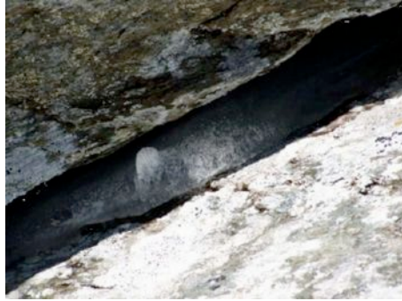
Figure 2.4: Ice-filled discontinuity (Image Courtesy of U. Morra di Cella).
