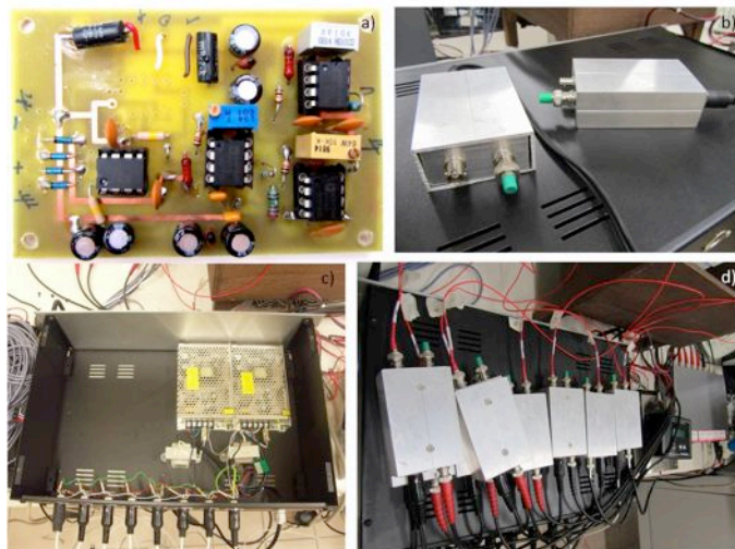
Figure F.1: Specifically designed and manufactured preamplifiers: a) amplifier circuit; b) shielding cases; c) power supply; d) connection between sensors-amplifiers and acquisition board (on the right).
