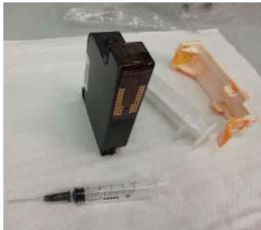
Figure 35. Ink-filled cartridge with precursor solution.
