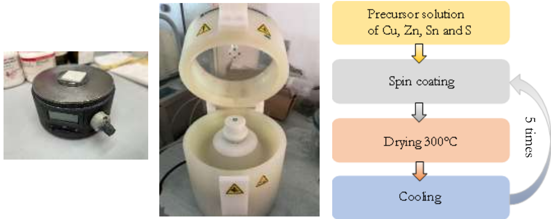
Figure 38. The two spin coating system used and the step of the process.
