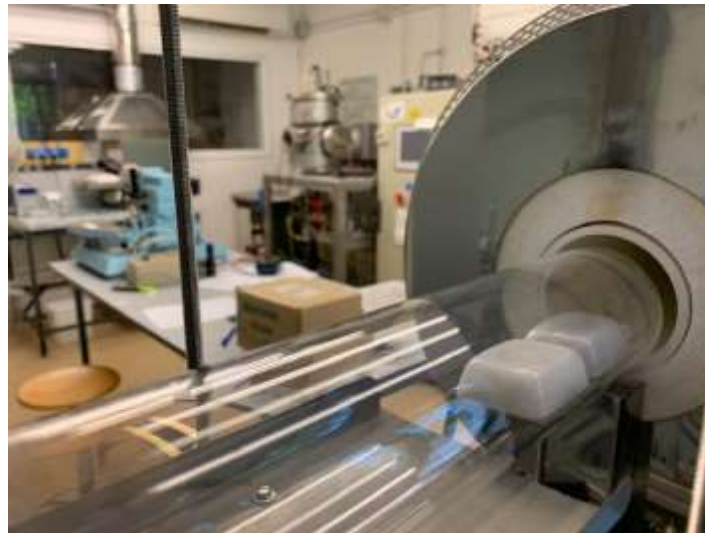
Figure 42. A detail of the annealing process, samples being cooled.
