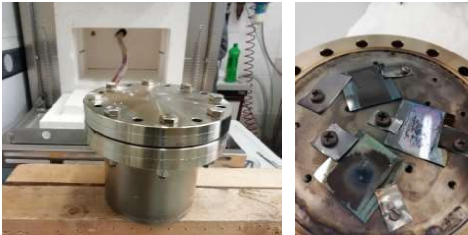
Figure 55. Home-made annealing chamber.
