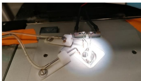
Figure 26. Experimental chamber for the measurements of cell fractional shortening and calcium fluorescence under imposed external pacing in a perfused Tyrode solution at constant temperature of 37°C.
