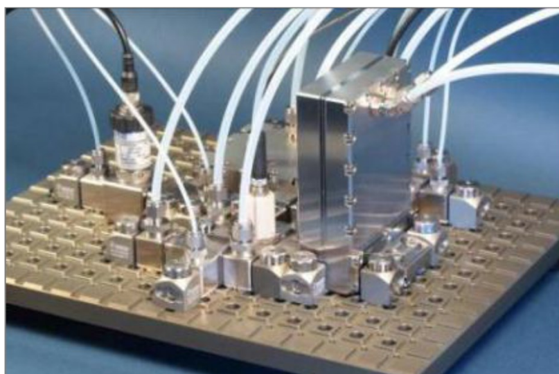
Figure 16 Automated continuous flow chemistry systems
