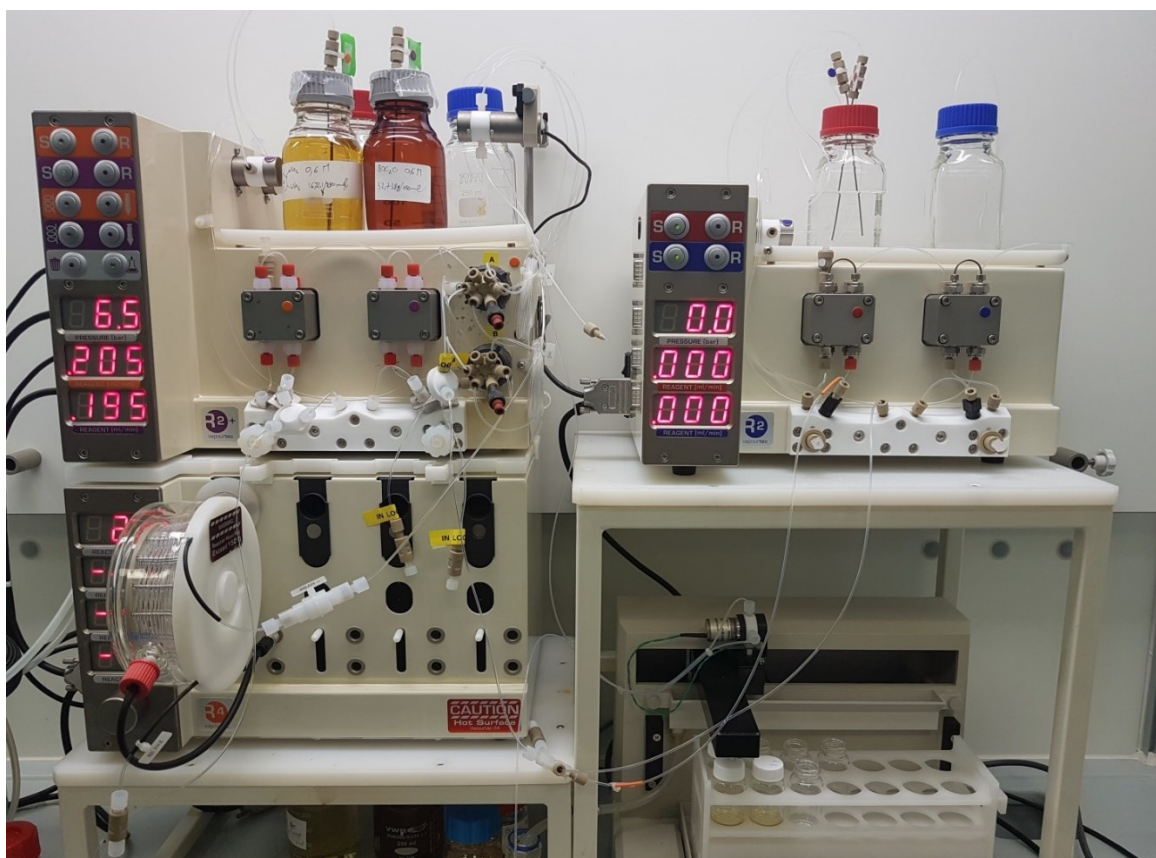
Figure 52 Flow reactor during the optimization
