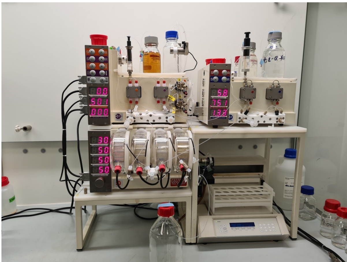
Figure 47 Flow reactor during step 3
