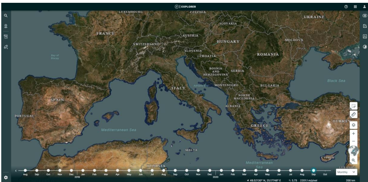
Figure 7: Graphical User Interface (GUI) of Planet Explorer. Through the graphical interface, users can select an area of interest, add filter parameters such as date range, cloud cover, satellite, and download the relevant satellite images
