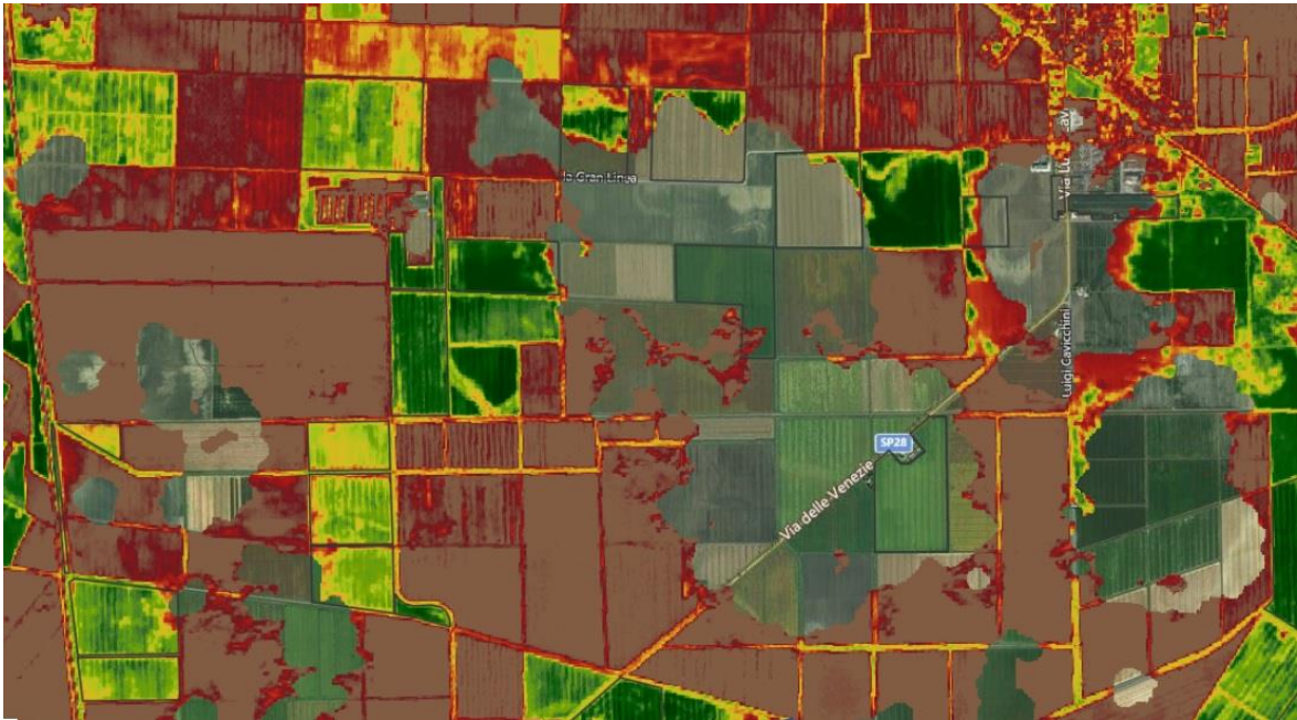
Figure 24: Modified soil-adjusted vegetation index (MSAVI) (date 11.04.2019) of the area of interest superimposed on a satellite base-map. The areas in which the MSAVI is not showed are cloud cover.
