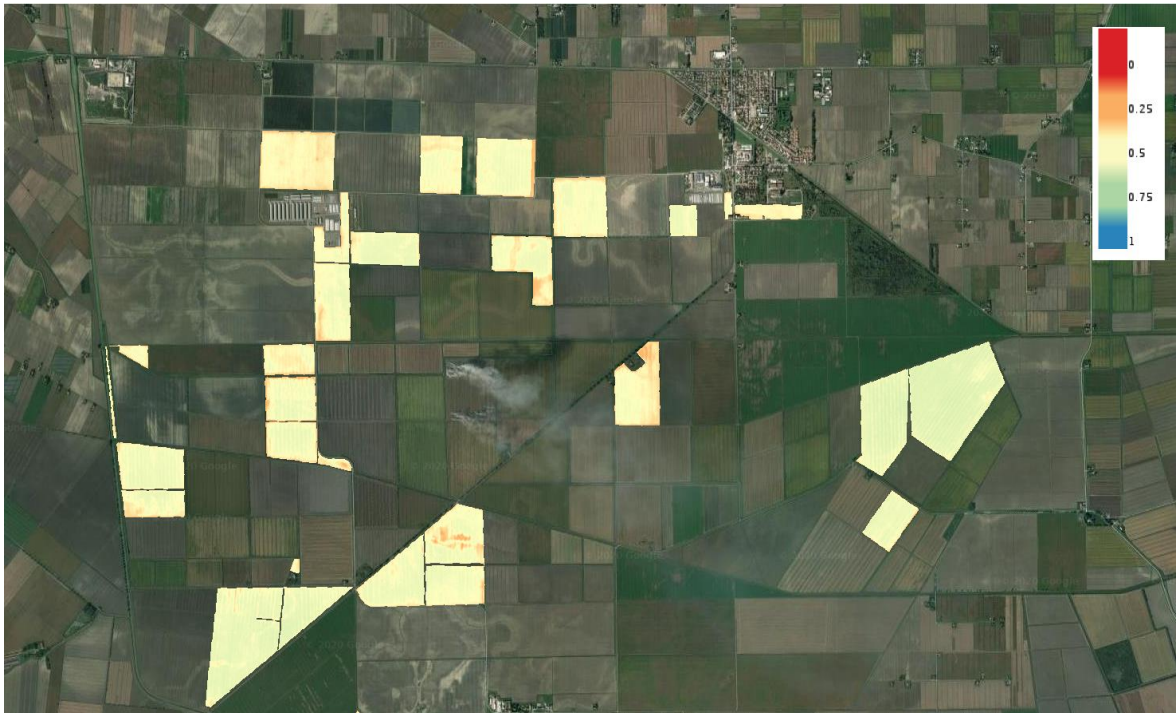
Figure 15: NDVI calculated for 27 fields, starting from PlanetScope (PS) data acquired on 15 May 2019, and superimposed on a Satellite base map.
