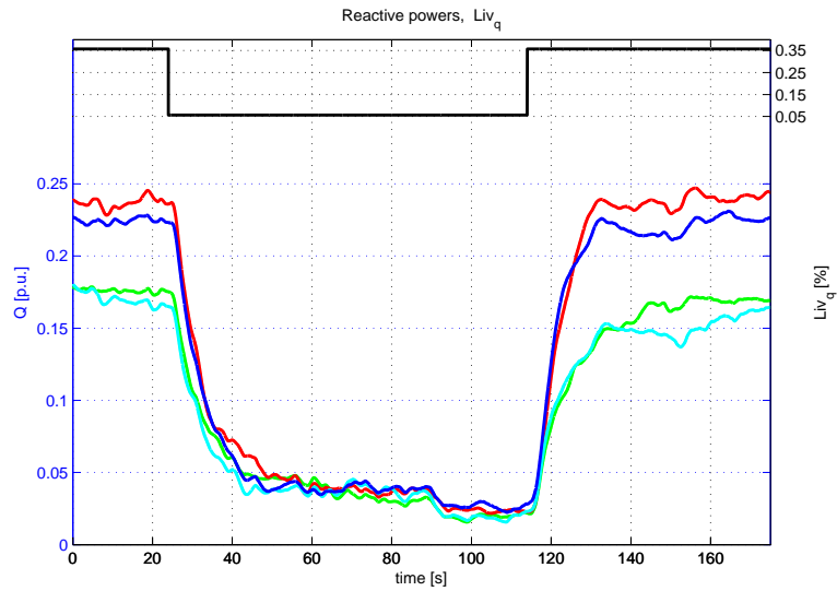
Figure 6.25: Case4 - Reactive power response - Reactive power response to a step of minus 0.3 in Liv q . Lines Red and Blue refer to the steam turbine generators while lines Green and Cyan refer to the gas turbine generators.
