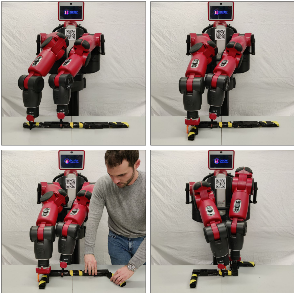
Figure 5.1 A Baxter robot executing actions in two domains involving the manipulation of an articulated object. A human can act on an articulated object's joint at any time, forcing the robot to re-plan.
