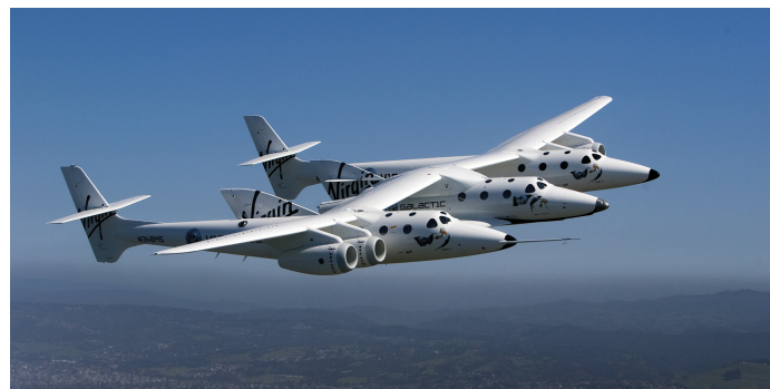
Fig. 2.34 SpaceShipTwo underneath its carrier aircraft the WhiteKnightTwo
