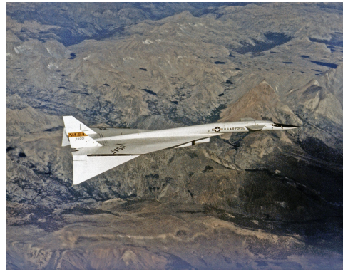
Fig. 2.17 XB-70 Valkyrie in supersonic flight configuration
