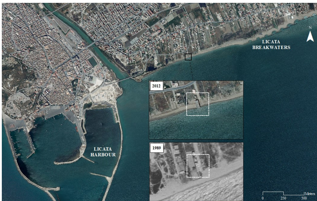
Fig. 66 – The area easterly the Southern Imera river mouth faced severe coastal erosion, holidays houses were compromised and partly submerged by sea water, as shown by the white squares that framed a house partly swallowed up by the sea.
