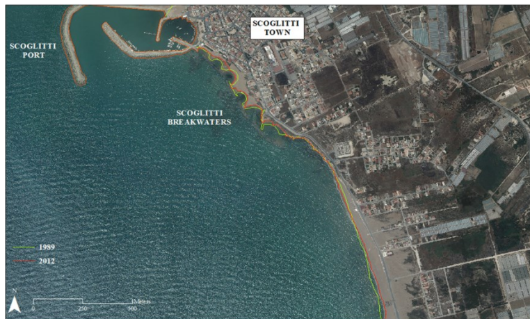
Fig. 56 – Sector n. 4 is southeasterly the Scoglitti port and is ca. 5,5 km long. The coastal evolution over the mid-term period (1989 – 2012) has been mainly affected by the port, any significant accretional phenomena have been detected even though 5 breakwaters have been replaced down-drift the port. However, the stability class is the most representative (61%).
