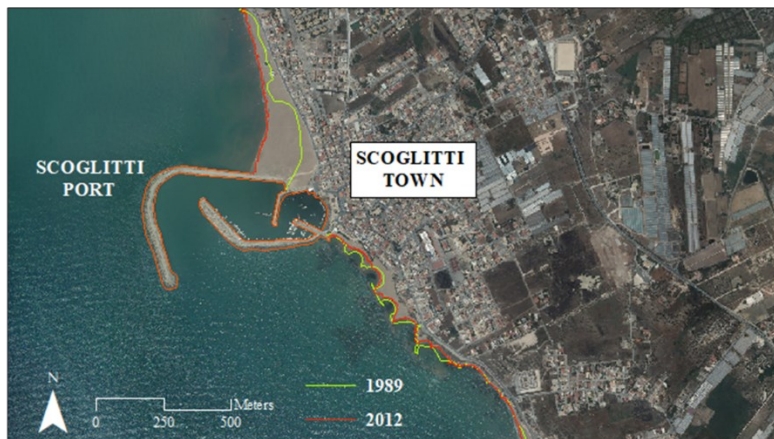
Fig. 55 – Sector n. 3 shoreline changes over the mid-term period (1989 – 2012), it is the longest sector by length (ca. 24 km). It mainly showed a stable trend (39%), as shown the histogram chart, even though it partly faced landward movements with the highest negative WLR value of -2,93 m/year. Very high accretion (8,31 m/year) occurred up-drift the northern dike of the Scoglitti port, finished in 2008, which worked as sediment trap.
