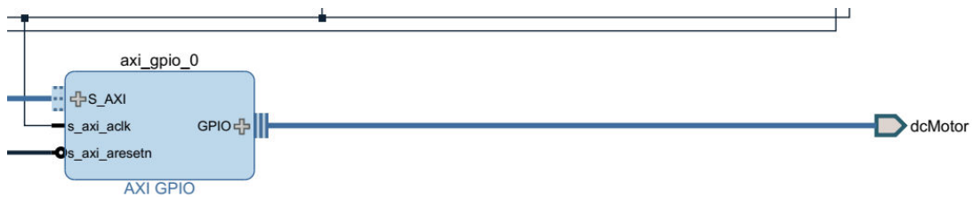
Figure 4.15: IP for Rotating the Tank.
