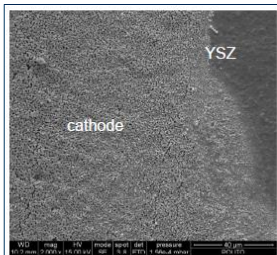
Figure 5-19: Top view of the LSM cathode/YSZ interface
