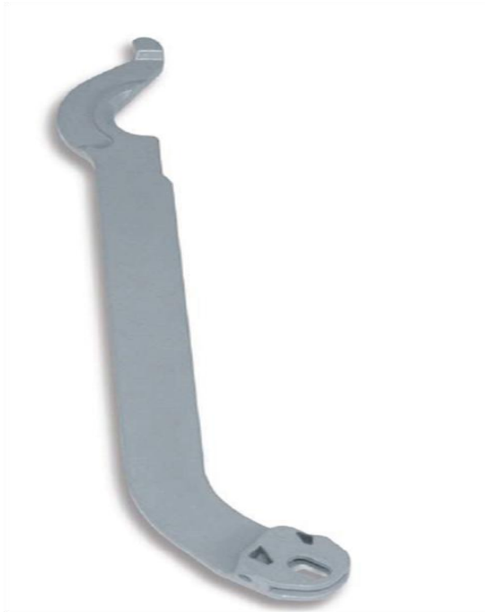
Figure 47: Supports for the table of plane's seats produced with UNIFONT-94 self-hardening aluminum alloy [70].
