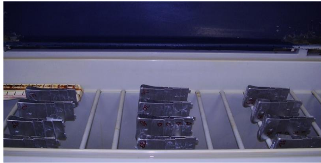
Figure 59: Position of the samples inside the batch during salt spray corrosion test.
