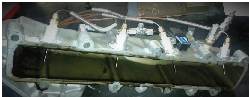
Figure 1.46: Picture of the intake manifold that shows the installation of the thermocouples.
