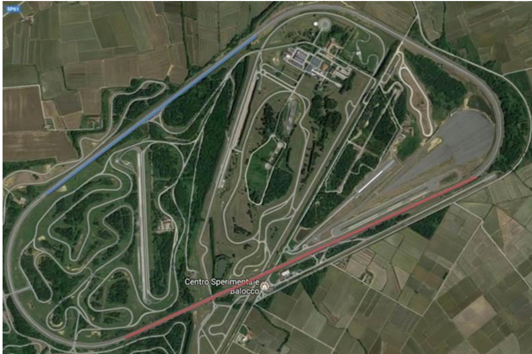
Figure 2.3: Test track (FCA Balocco Proving Ground), with highlighted the two straight sectors where the coast-down tests have been performed.
