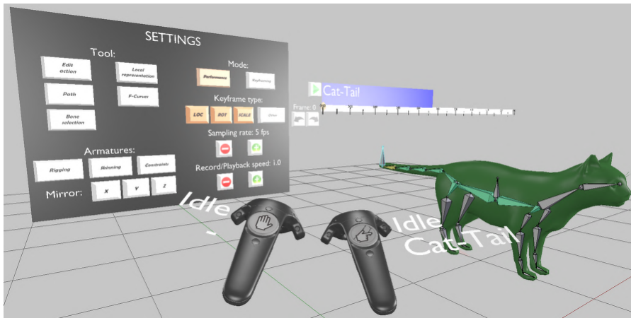
Figure 3.7: First-person view of the new VR Blender interface. The Settings panel includes the new widgets introduced to manage armature deformation-based animation tasks.
