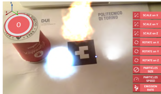
Figure 4.11: The T4T interface in tuning mode. Parameters of selected object can be tuned by manipulating the tangible prop acting as a control knob.
