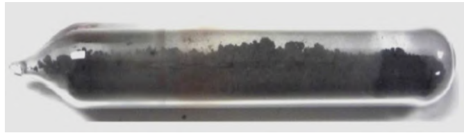
Fig. 3.2: FeSe_{0.5}Te_{0.5} reacted powders, in a pyrex glass tube.
