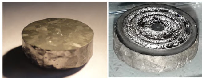
Fig. 3.4: FeSe_{0.5}Te_{0.5} target as prepared and after many depositions
