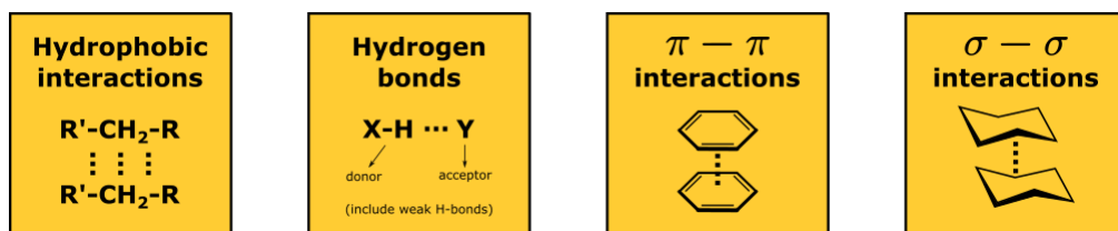
Fig. 1.2 Main intermolecular interactions classes which drive the self assembly process. Hydrophobic interactions exist between hydrocarbon chains or similar nonpolar regions of a large molecule. Hydrogen bonds form between atoms having a large difference in electronegativity. Most of the times, the donor is usually a Hydrogen atom and the acceptor is one amongst N, O, and halogens; a wide range of bond strengths are possible depending on solvent and the specific functional group combinations. \pi - \pi and \sigma - \sigma are weaker interactions compared to the previous ones, and originate from the interaction of the electronic orbitals of the \pi -bonds and \sigma -bonds respectively.
