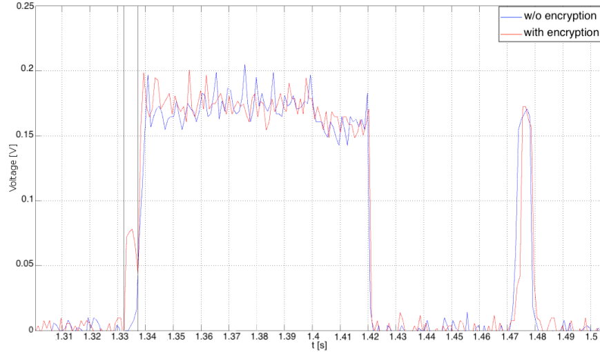
Figure 63: Voltage samples corresponding to a single packet transmission, with and without encryption.
