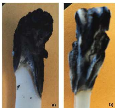
Figure 3.2.3.2.2: LOI residues of the sample (a) EVA/Hy and (b) EVA/Hy/10Sil.
