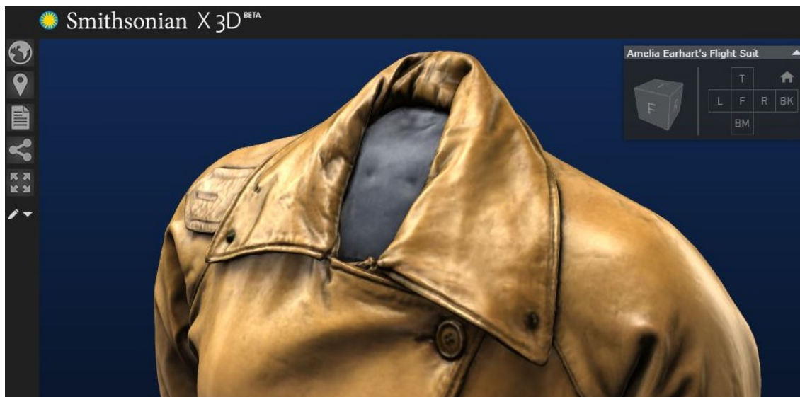
Figure 2.9: Smithsonian X3D [Smi11] is an example of 3D Web viewer using the ViewCube interface component (in this case presented at the top right corner of the 3D rendering window). The 3D cube widget rotates synchronously with the 3D model; it has the primary purpose to provide the final user with a feedback on the orientation of the 3D scene. The component can be used also to directly drive the scene interactions (by rotating the 3D cube the final user applies a corresponding rotation to the 3D scene).
