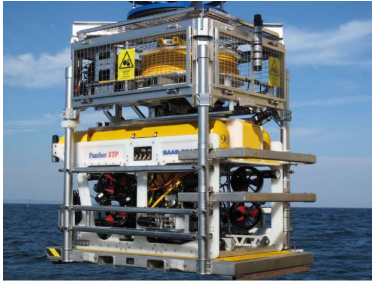
Figure 2.4: Panther XT Plus ready in its TMS. The Panther-XT Plus is a 1000 m rated ROV fitted with ten 500 VDC thrusters (eight horizontal and two vertical). It can be used as a free swimmer or in conjunction with a TMS. Image from http://www.saabseaeeye.com
