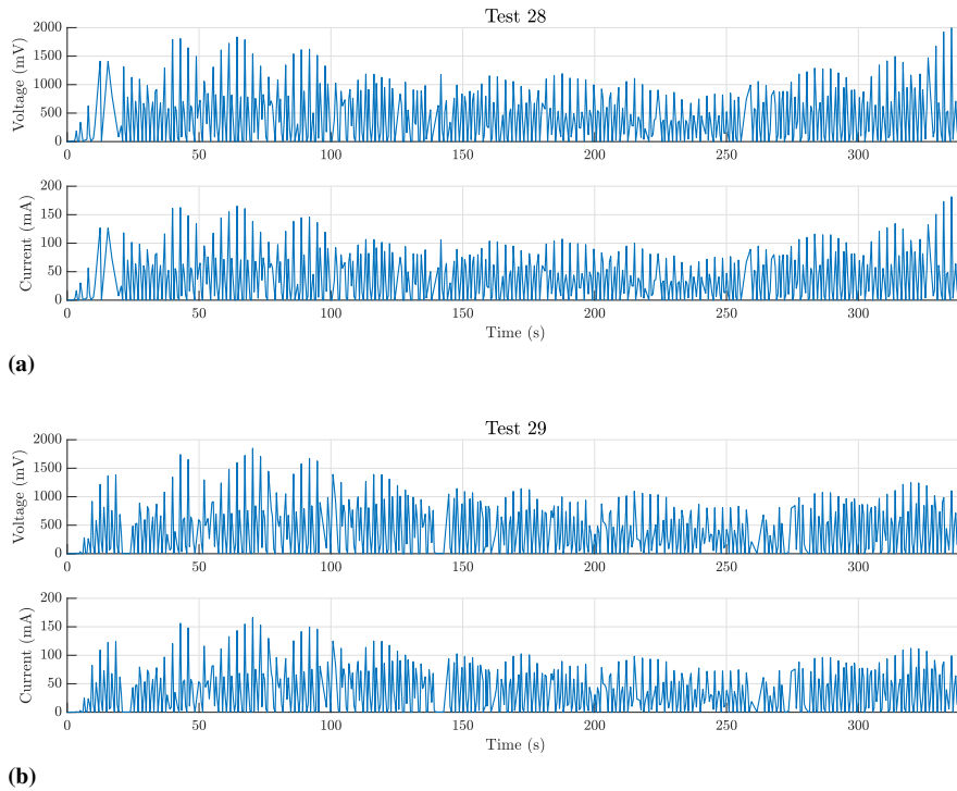
Figure 4.11: Generated voltage and current by the WAVE harvesting system for test no. 28 (a) and no. 29 (b).
