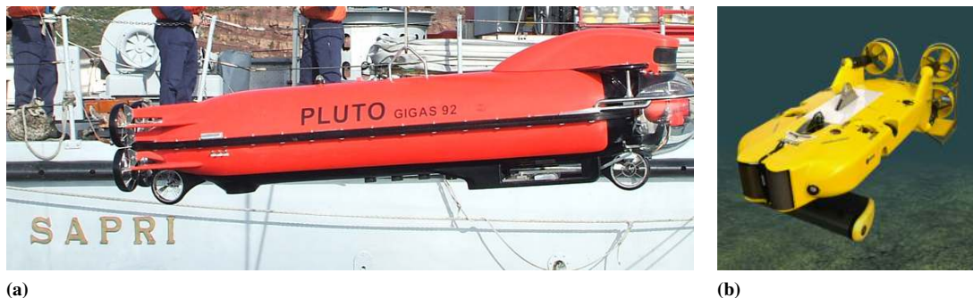
Figure 2.5: Two examples of ROVs largely used in the Navy community for mine identification and disposal up to 600 m. (a) The Pluto Gigas ROV, manufactured by idRobotica ( http://www.idrobotica.com/pluto-gigas.php ), while deployed from an Italian Navy Mine Hunting Vessel. (b) The Saab Double Eagle MKIII ROV ( https://saab.com/naval/underwater-systems/remotely-operated-vehicles/double_eagle_mkii_iii/ ), with its rotatable multi-frequency sonar for detection and classification of mines.
