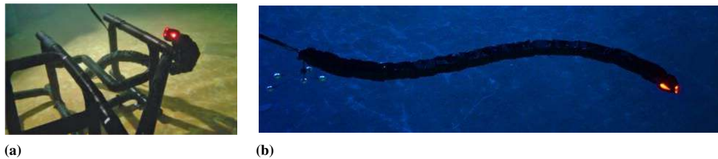
Figure 2.7: The underwater snake robot Mamba implemented the at Norwegian University of Science and Technology. (a) Mamba moves inside a dummy underwater structure. (b) Mamba in the pool with the markers attached on the tail for position measurements.
