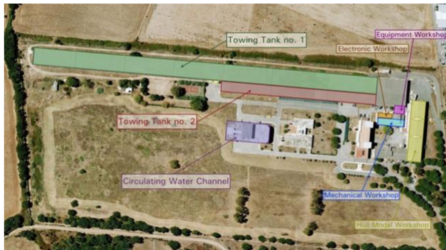
Figure 4.1: Overview of CNR-INSEAN test facilities. The Towing Tank no.2 (in red) was used for testing the WAVE module ( http://www.insean.cnr.it/ ).
