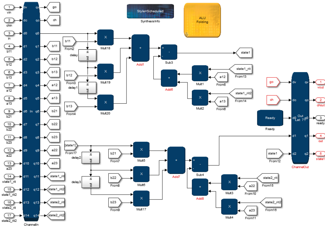
Figure 4.5: Implementation of the filter in the Intel DSP Builder tool.
