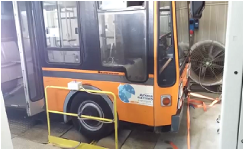
Figure 5.9: Photograph of the minibus during a test session on the chassis dynamometer.
