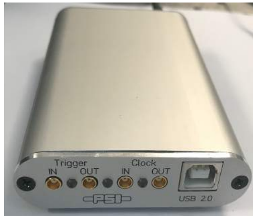
Figure 22: PSI DRS4 evaluation board.
