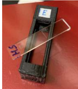
Figure 53: Silver activated phosphate glasses samples.
