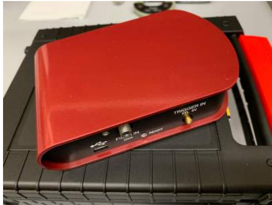
Figure 45: The CCS200 spectrometer from Thorlabs.
