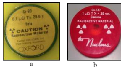
Figure 20: (a) Radioactive source \text{Sr}^{90} , (b) \text{Cs}^{137} used in beta detector measurements.
