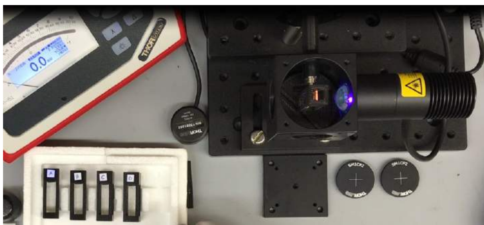
Figure 64: The complete and compact first prototype to acquire the RPL signal from the samples.
