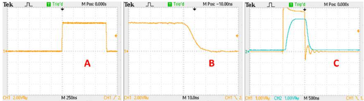
Figure 52: (A) Shape of a 1 \mu s pulse generated by a GPIO pin of the microcontroller; (B) Fall time of the TTL signal generated from the microcontroller; (C) Shape of the LED driving signal on the output of the MCP1407 (yellow line) and shape of the light signal detected by the SiPM LynX Module (light blue line).
