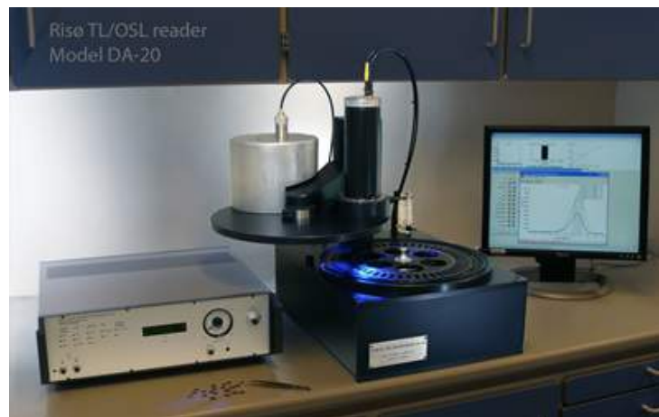
Figure 33: Risø Reader of the Nutech DTU.
