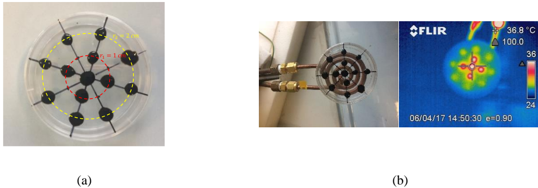
Fig. 1.14 (a) Magnetic nanoparticles drops on the top of a Petri dish (diameter 6 cm, height 1.3 cm). The two highlighted circumferences present a radius of 1 cm and 2 cm, respectively. (b) Experimental set-up (on the left) and temperature map of the surface of the petri dish after 40 seconds from the exposure start (on the right). Again, the targeted distribution of the magnetic field is well evident.
