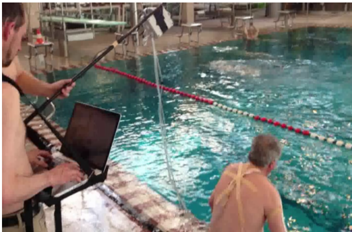
Figure 4.5. The test setup, with the waterproof-box fixed on fishing rod, notebook on hawker's-tray and tape-fixing of tubes on back of test person.
