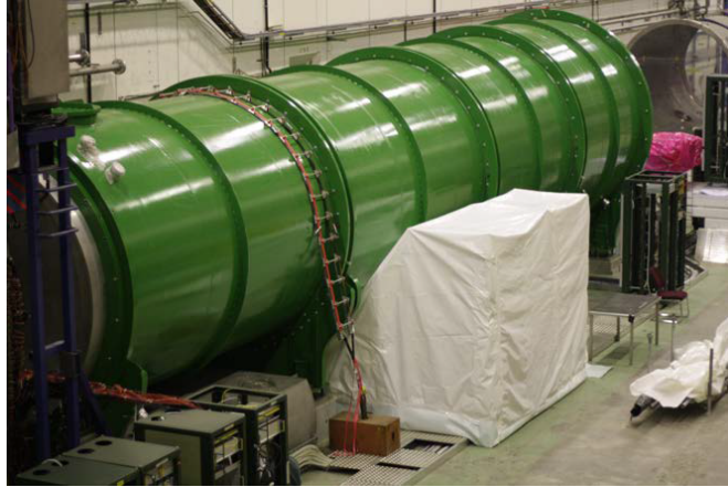
Figure 2.17: A picture of the RICH installed in the NA62 cavern.
