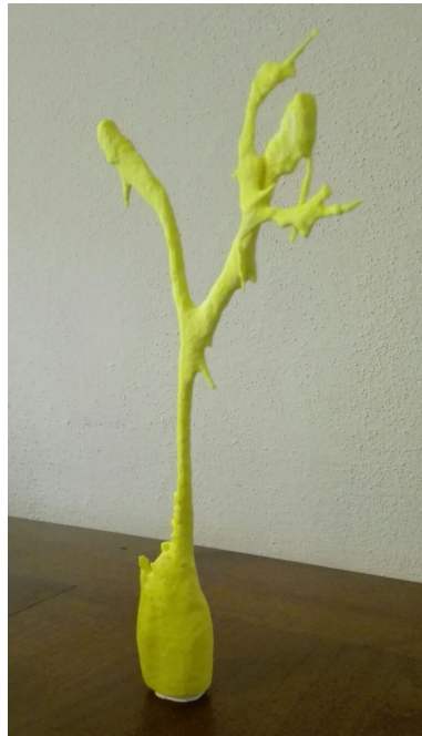
Figure 3.14: A Purkinje cell 3D-printed using a Stratasys Fortus 450mc (Stratasys)
