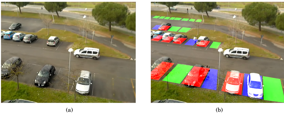
Figure 4.7: Example of parking lot analysis: background model at time t (a) and real-time output at time t (b).
