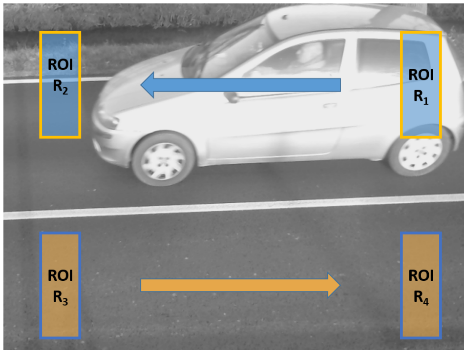
Figure 4.8: Traffic flow analysis: view from sensor test set-up and example of vehicles transit in the field of view of the sensor, which may cause occlusion to the upper lane.
