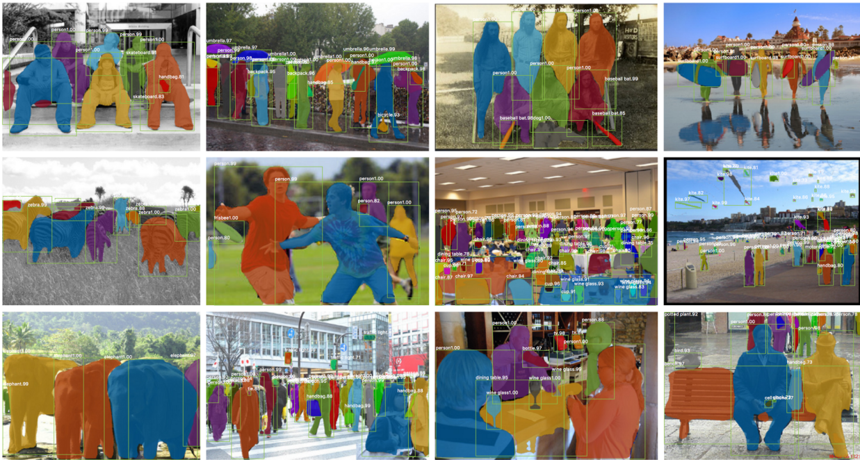
FIGURE 5.1: Example bounding boxes and predicted classes using the Mask R-CNN network [66]. Each segmented object is colored with a different color and a label is associated to the surrounding bounding box.
