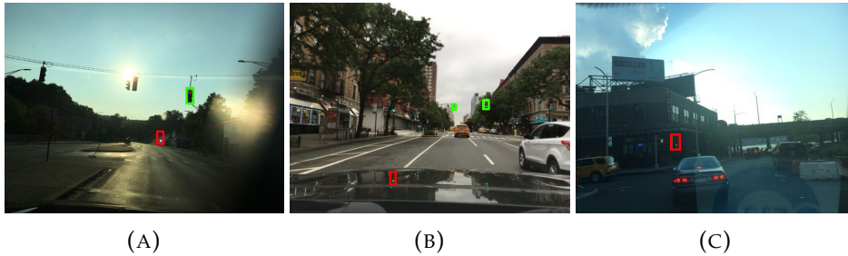
FIGURE 8.7: Failure modes of the presented method. When not enough data from a particular location are provided both (a) false negative detections due to the undetected objects or (b) temporarily consistent wrong detections can manifest. The largest challenge is (c) consistent and repeated detections of a objects that look similar to a traffic light over a period of time.
