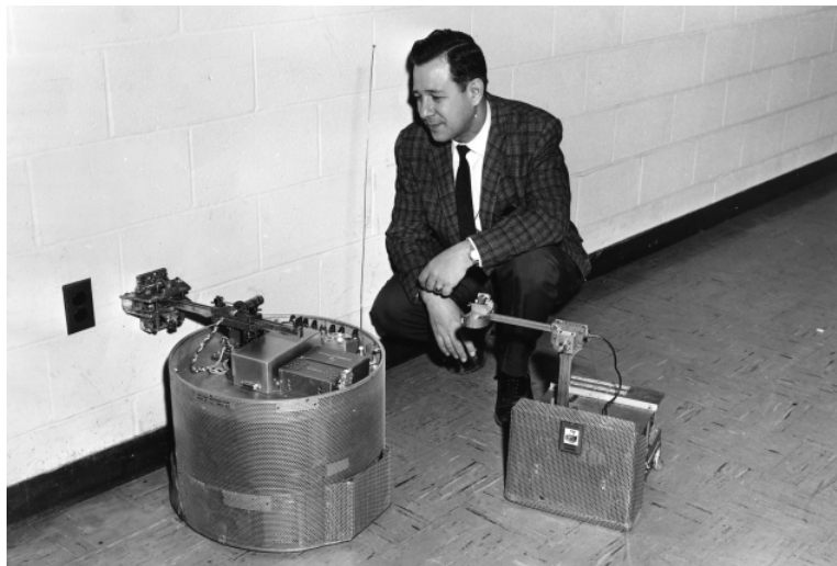
FIGURE 2.1: An image showing the autonomous rover built by the APL group in 1964 1 .
