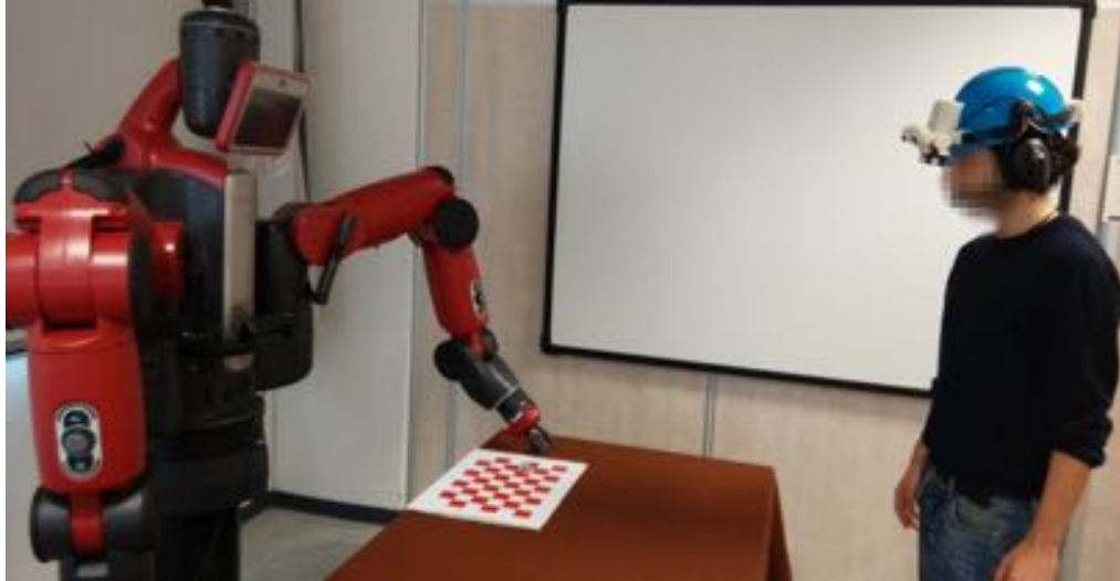
Figure 4.7: Experimental environment with Baxter and operator wearing the HUD.
