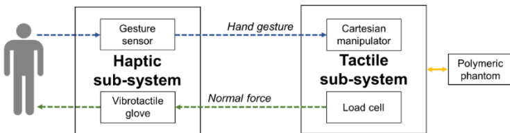
Figure 59: Block diagram: bidirectional data streaming between the haptic and tactile sub-systems provided via UDP: the optical controller conveyed speed and position of the centre of mass of the user's hand from the first environment to the Cartesian manipulator in the remote one (blue arrow) and, while sliding, normal force data collected by the load cell from the platform to the vibro-tactile glove to deliver the spike-based stimulation (green arrow).
