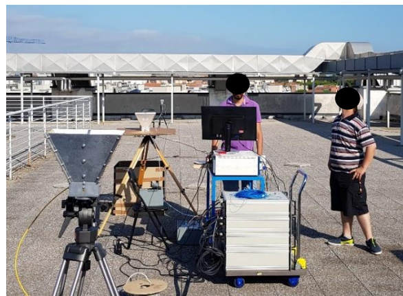
Figure 4-8: On-field deployment of the photonics-based 2TXs x 2 RXs MIMO radar network
