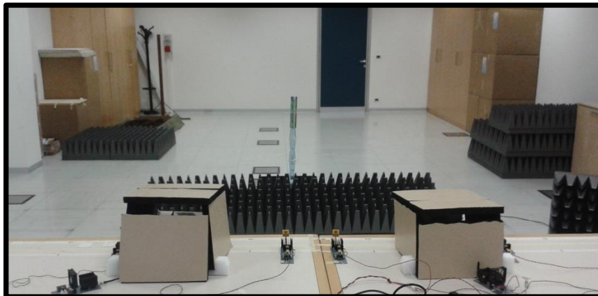
Figure 4-36: 2TXs x 4 RXs MIMO experiment indoor test layout
