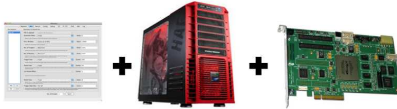
Fig. 35 - Emulation system: GUI, Workstation and Development board.
