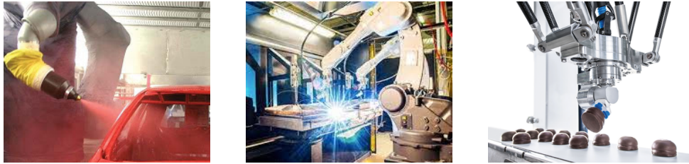
Figure 2.1: Position control is widely employed in applications that do not involve contact forces between the manipulator and the environment, as spray painting, spot welding, and pick-and-place tasks.
