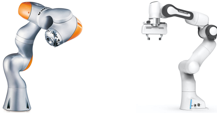
Figure 2.3: On the left KUKA LBR iiwa 14 robotic arm, on the right Franka Emika Panda manipulator. LBR stands for “Leichtbauroboter” (German for lightweight robot), and iiwa for “intelligent industrial work assistant”.
