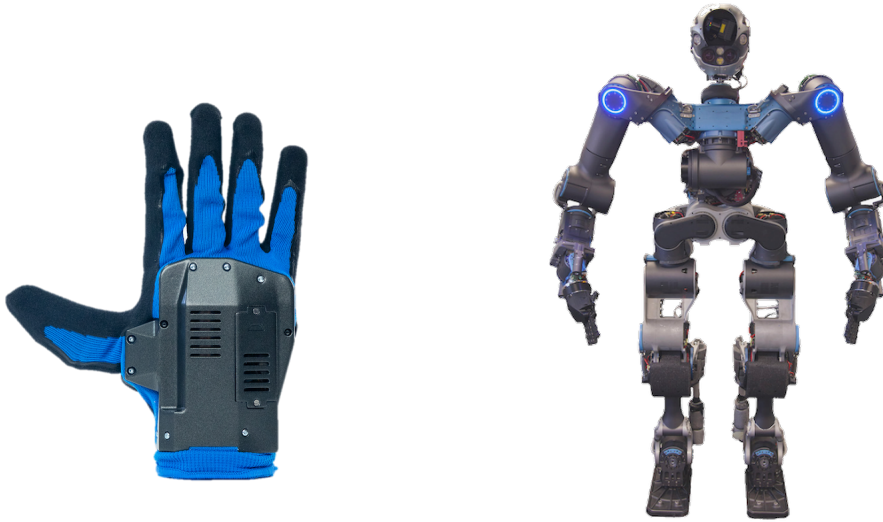
Figure 2.5: Left: the Pisa/IIT SoftHand simplifies grasp planning and control, through its synergy-driven design. Right: the humanoid robot WALK-MAN.
